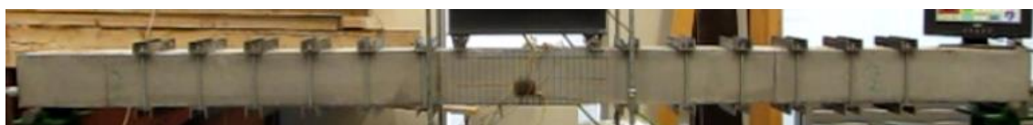
Figure 2. External stirrups on two extra beams of Model type 2, with length of 3860 mm.
